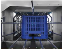
Side and upper guides with quick and easy adjustment
